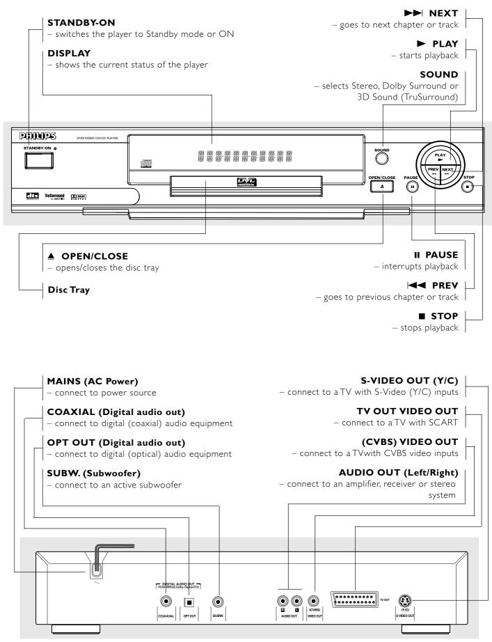
Caution: Do not touch the inner pins of the jacks on the rear panel connectors. Electrostatic discharge may cause permanent damage to the unit.
